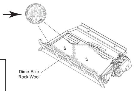
Figure 19 - Placing Rock Wool
